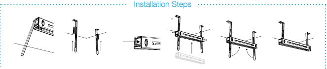
\*Fire Fastener needed when used channel-side up ('u' orientation). Tested at ambient temperatures, contact Gripple for full product information, submittal data and technical support \*\*When installed correctly, button must be fully retracted and flush with the cartridge edge. Do not adjust under load. SWL is dependent on the bracket size and orientation.
