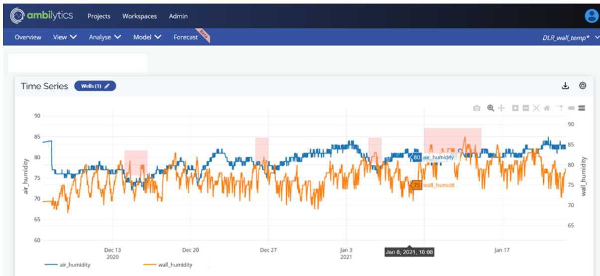
Figure 4 – Lack of Correlation between Air & Wall Humidities (High Likelihood of Mould Growth & Potential Structural Issues)
